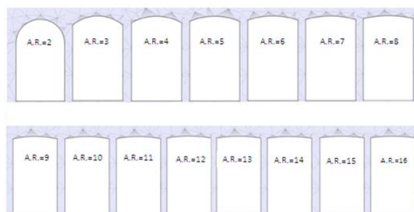
Figure 1. The modeling of vaulted tunnels with width of 4 meters and different arch radius (A.R. is arch radius of tunnel to meter)
